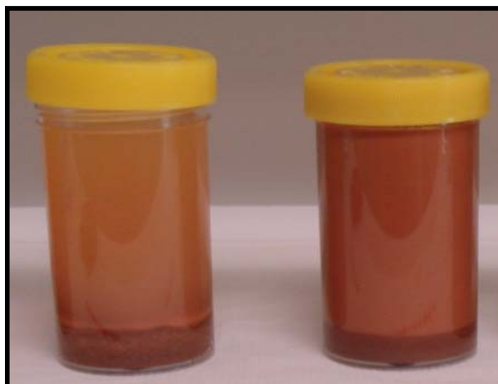
Figure 2. Clay dispersion in response to an exchangeable potassium percentage of 40% (right) or exchangeable sodium percentage of 40% (left).
